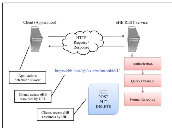
Figure 2. The architecture of the eHB software service and its interaction with client systems.
